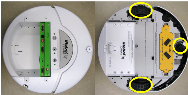
Figure 2. iRobot Roomba, with underside view: two-wheel base and caster highlighted.
