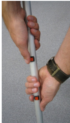
Figure 9. Broomstick-Roomba interface, with mounted buttons.
